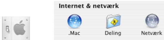
2. Select **Ethernet (INDBYGGET ETHERNET)** and click **Configure (KONFIGURER)**. If you also have a network at home, it might be a good idea to create a new location so you can easily switch between network settings.
